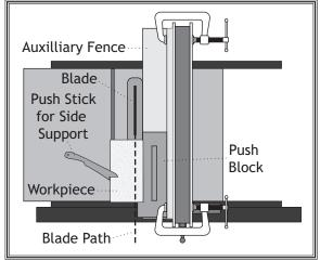
**Figure 79.** Setup in preparation for ripping.
